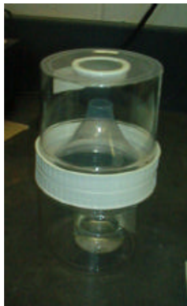
Figure 2 - Lab container for mosquito larvae with mosquito collection jar in bottom half of container
